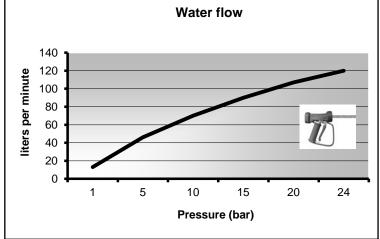
water flow in I/min with totally pulled trigger
